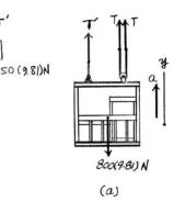
**Equations of Motion:** Using the result of **a** and referring to the free-body diagram of the hoist and block shown in Fig. *a*,
